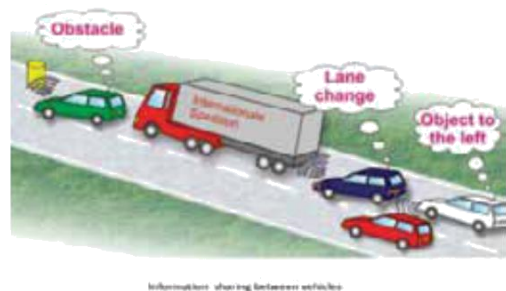
Fig.3 Vehicle to vehicle (V2V) Communication
