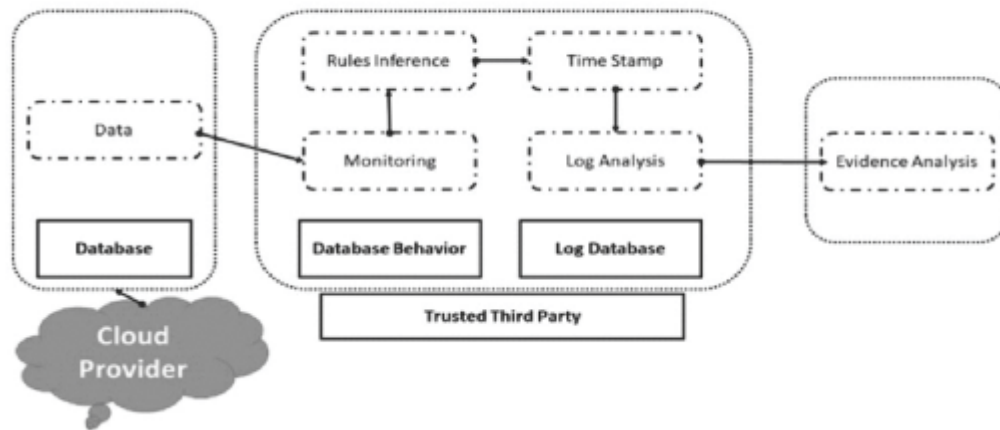
Fig 5: Evidence Collection Proposed Framework
